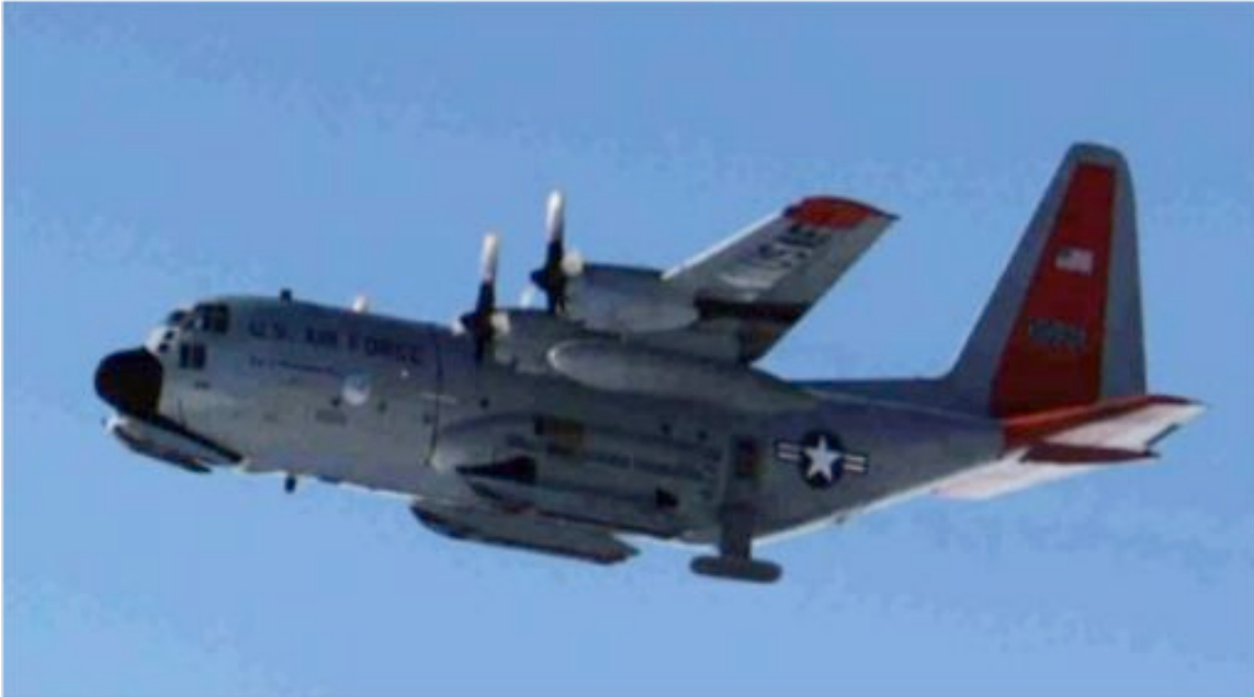
Figure 1: An LC130 operated by the New York Air National Guard. Our instruments are in the pod hanging below the air force star.
